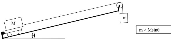
Determine the theoretical energy equation in variable form for a cart traveling up the inclined plane above. The cart starts from rest and the mass is allowed to fall a height of h. Do not include any corrections for friction or rotational energy. All work including a diagram should be attached.
