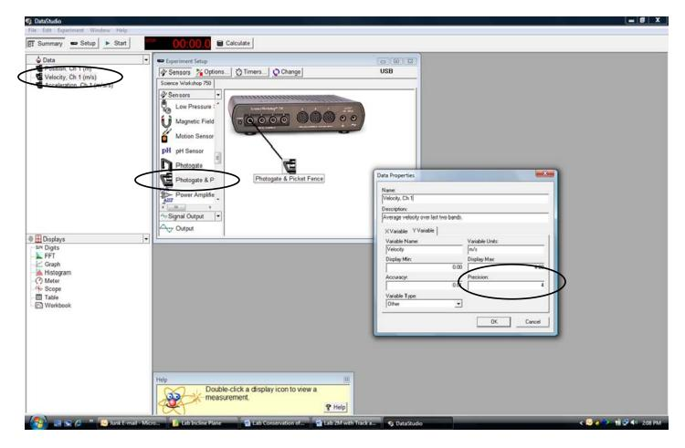
Now double click on the Photogate & Picket Fence icon that is connected to your virtual interface box. Under the *Constant* tab in the window that appears, change the constant to 0.010 m. This is the spacing between the leading edges of the bands on the PF.
